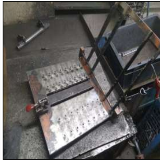
Fig.1 Spatter observed in Nut & Bush of K4 frame Battery Bkt. Part More than 30% rework of battery bracket / day.
