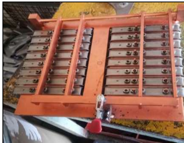
Fig.5 Development of Tack Welding Fixture
